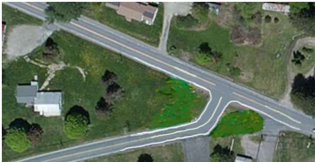
Photo 7: Revised photo showing the intersection of NY 43 with Garfield Road with a right angle.
