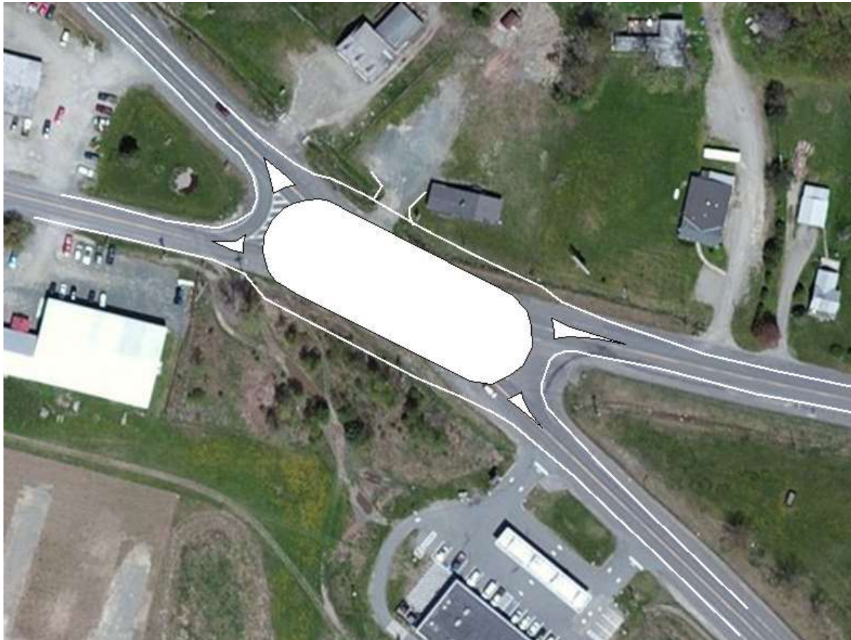
Photo 6: Intersection of NY 22 & NY 43 shown with a roundabout treatment. Due to skewed angle of intersection, a circular roundabout would not work at this intersection due to the required entrance angles.
